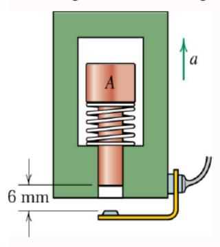
Specify the neccessary spring stiffness k which will permit the plunger to deflect 6 mm beyond the equilibrium position and touch the electical contact when the steadily but slowly increasing upward acceleration reaches 5g. Friction may be neglected. Ans: 818 N/m
