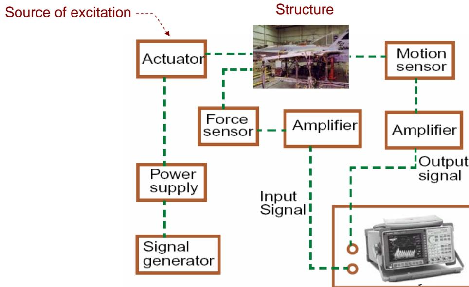
**Dynamic signal analyzer:** display both time and frequency responses and real time calculation of Fourier transform.
