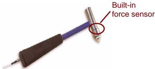
provides impulsive force to the tested structure
