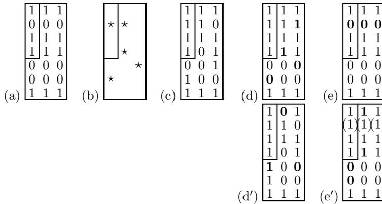
Figure 11.6. A product code. (a) A string 1011 encoded using a concatenated code consisting of two Hamming codes,  $H(3, 1)$  and  $H(7, 4)$ . (b) a noise pattern that flips 5 bits. (c) The received vector. (d) After decoding using the horizontal  $(3, 1)$  decoder, and (e) after subsequently using the vertical  $(7, 4)$  decoder. The decoded vector matches the original. (d', e') After decoding in the other order, three errors still remain.
