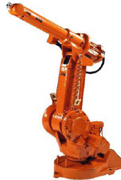
Figure 1.9: The ABB IRB1400 Robot, a six-DOF elbow manipulator (right). The symbolic representation of this manipulator (left) shows why it is referred to as an anthropomorphic robot. The links and joints are analogous to human joints and limbs. (Photo courtesy of ABB.)
