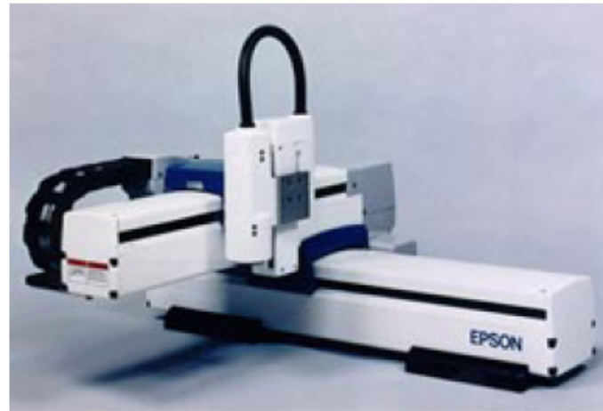
Figure 1.16: The Epson Cartesian Robot. Cartesian robot designs allow increased structural rigidity and hence higher precision. Cartesian robots are often used in pick and place operations. (Photo courtesy of Epson Robots.)
