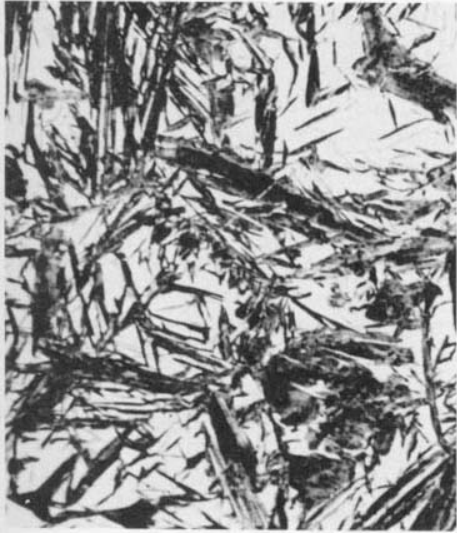
Figure 10.13 Photomicrograph showing the martensitic microstructure. The needle-shaped grains are the martensite phase, and the white regions are austenite that failed to transform during the rapid quench. 1220x. (Photomicrograph courtesy of United States Steel Corporation.)
