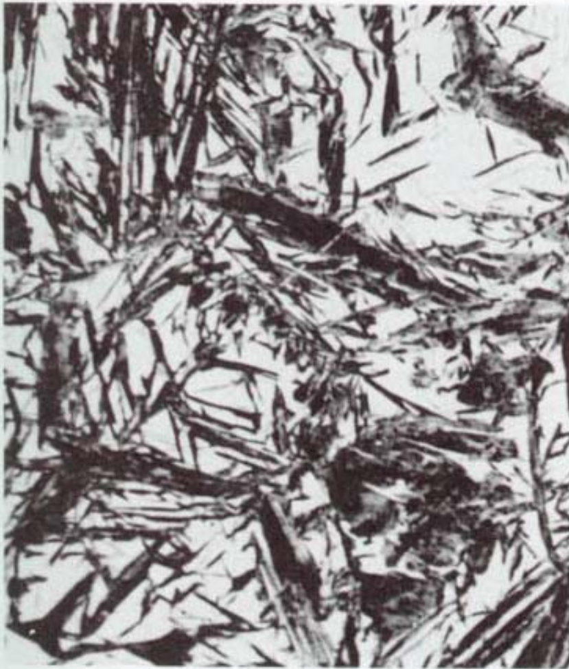
Figure 10.13 Photomicrograph showing the martensitic microstructure. The needle-shaped grains are the martensite phase, and the white regions are austenite that failed to transform during the rapid quench. 1220 \times . (Photomicrograph courtesy of United States Steel Corporation.)
