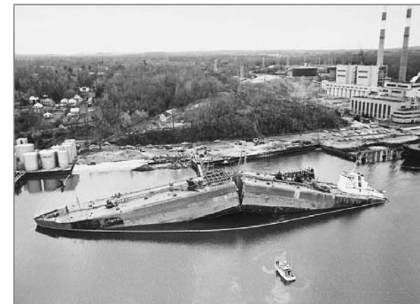
An oil tanker that fractured in a brittle manner by crack propagation around its girth. (Photography by Neal Boenzi. Reprinted with permission from The New York Times .)
