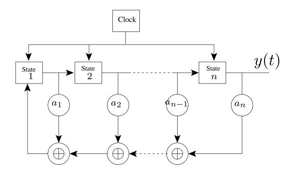
$$x(t+1) = \begin{bmatrix} a_1 & a_2 & \dots & a_n \\ 1 & 0 & \dots & 0 \\ \vdots & \ddots & & \vdots \\ 0 & \dots & 1 & 0 \end{bmatrix} x(t)$$
