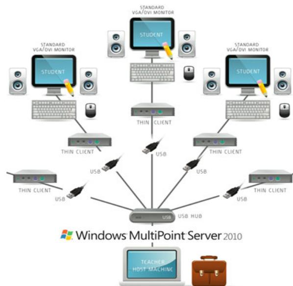
Figure 2. Connectivity of Multi-point scheme
