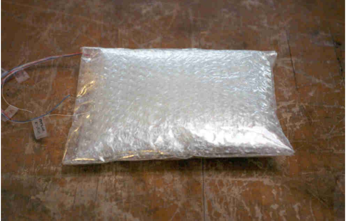
Figure 5.4: The adaptive wood composite sample covered by 8 layers of bubble wrap.
